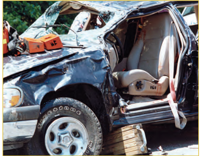
The roof crushed down to the seat.
